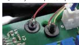
Example or probe with the double-sided tape
